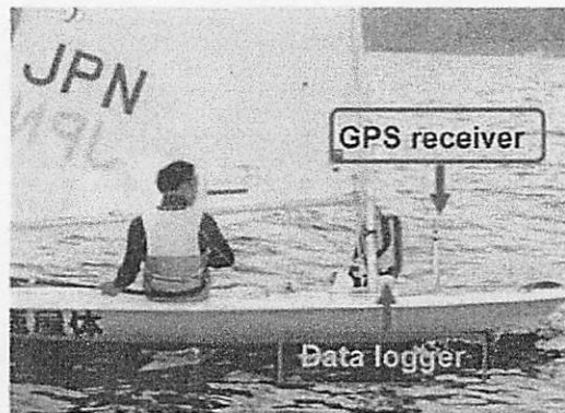
Figure1 A high-performance differential global position system (GPS) unit (Crescent A100, 20 Hz, Hemisphere) was placed in the bow of the boat to measure boat speed
